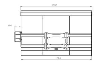
Loading capacity: 1,4 m<sup>3</sup> Spreading wide: **5-6 m** Net weight: 500 kg Gross weight: 550 kg
