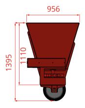
Loading capacity: **1,2 m³** Spreading wide: **4-6 m**
